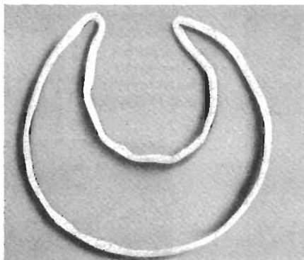
Fig. 2. Transmitting coil has been shaped to form L1 and L2.
