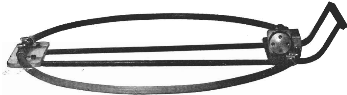
Locator drags easily from line attached to boat. Note round magnet on oscillator box, used to turn unit on and off.
