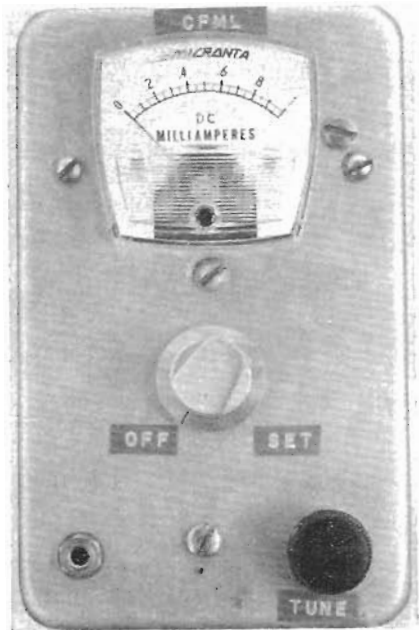
Fig. 5—A meter and only two controls is an indication of the locator's simplicity and ease of operation. The jack at lower left is for the audible monitor.
