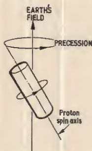
Fig. 2 Precession of proton relative to earth's field when acted upon by external magnetic influence
