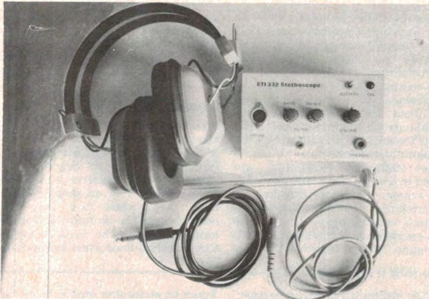
Completed stethoscope, ready for action! The probe here was made from a crystal earpiece, a length of 10 mm tubing being pushed over the ear plug.
