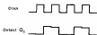
Fig. 6. Shows how the output of the 1.4kHz binary oscillator is affected by the clock generator. The steps in the waveform are removed by a clamping circuit.
