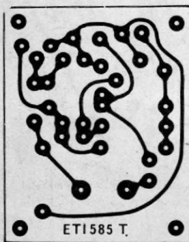
Fig. 7. Printed circuit board of transmitter. Full size 46 x 36mm.
