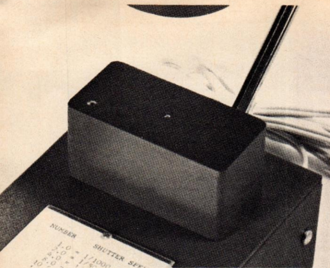
Fig. 4. Details of the camera mounting block. The two photosensitive devices (Q2 and LDR1) are mounted close to the upper surface of the block.
