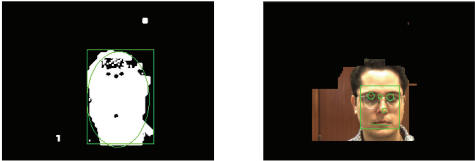
Fig. 4. Skin color detection using depth information.
