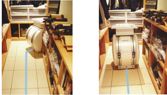
Fig. 8. Robot in movement, guided by line-marker
