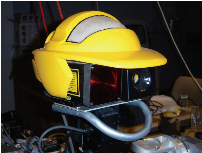
Fig. 5. Robot head includes camera, laser pointer and five LEDs.
