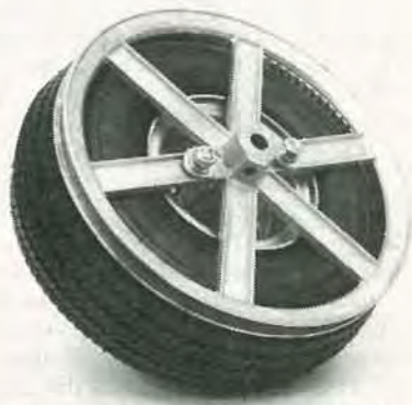
FIG. 7—IF BOLTED TOGETHER PROPERLY, the wheel and pulley assembly will resemble the one shown here.
