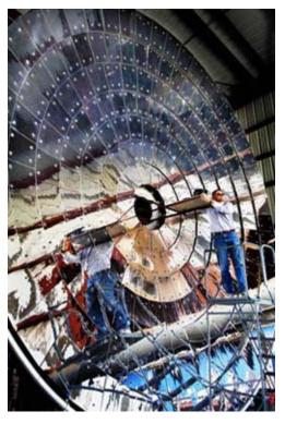
Sandia researcher Rich Diver checks out the solar furnace which will be the initial source of concentrated solar heat for the CR5 prototype. Eventually parabolic dishes will provide the thermal energy. (Photo by Randy Montoya)
