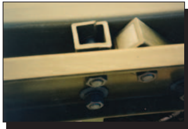
Figure 36—This tube cracked when bolts were overtightened on one of the bridges being tested at the Forest Products Laboratory.
