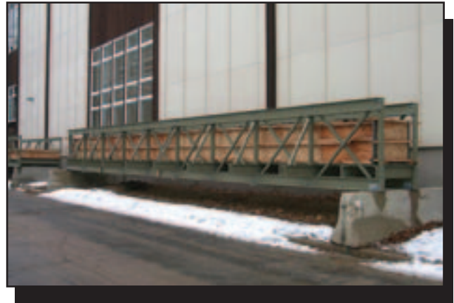
Figure 33—Two FRP bridges—one 22 feet long (left) and the other 44 feet long (right)—were tested at the Forest Products Laboratory in Madison, WI.
