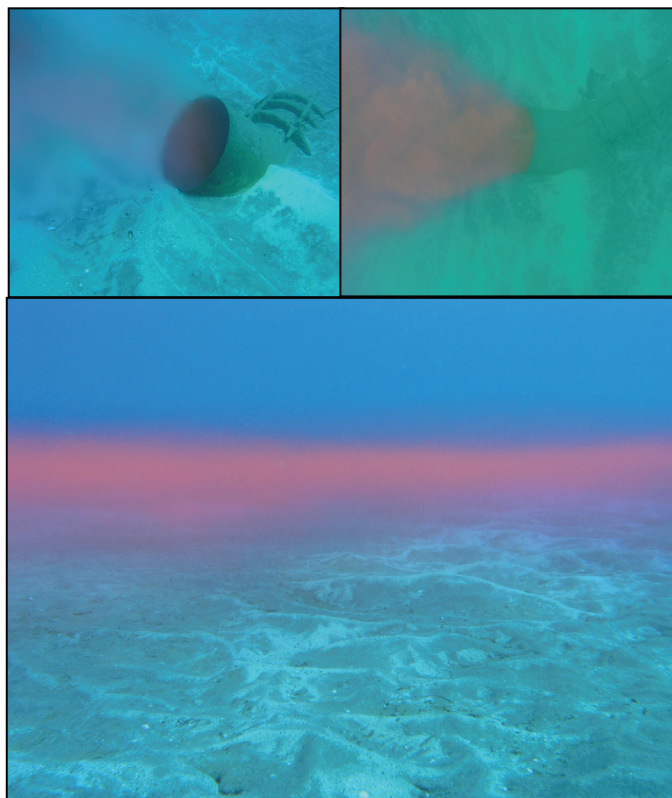
Fig. 2. Pictures from an ad hoc brine discharge dyed by rhodamine in Maspalomas beach. Near (upper panel) and Far field (lower panel) regions can be observed.
