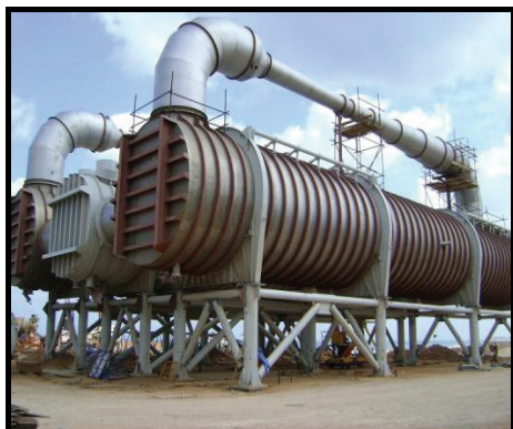
(a) Circular vessel evaporator.
