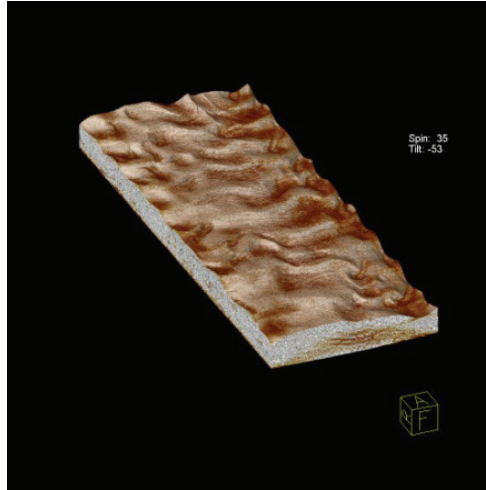
Fig. 2. Three-dimensional X-ray image of a sediment bed 300 mm wide by 300 mm high by 900 mm long, formed from 1500 slices of 512 x 512 pixels.
