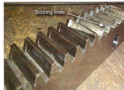
Shown here is a classic example of a scoring failure, which occurs when there's not enough lubrication to create a film between the teeth of the rack and pinion. Careful!
