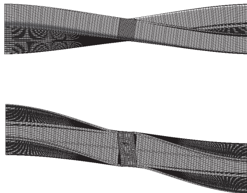
Fig. 12. Deformation of segmented pontoon, lateral and bird view
