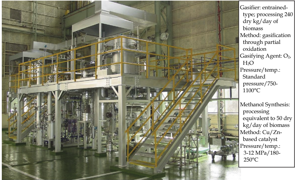
Fig. 8. "Norin Green No. 1", a test plant of gasification and biomethanol production, located in Nagasaki Research & Development Center, Mitsubishi Heavy Industries Ltd, Nagasaki, Japan.
