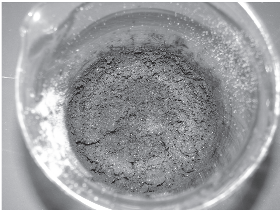
Fig. 17. Mid-value or low-value fractions from DDGS (such as fiber) can be thermochemically converted into biochar, which can subsequently be used to produce energy, fertilizer, or as a precursor to other bio-based materials.
