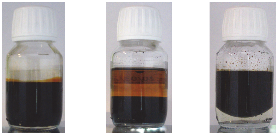
Fig. 5. Pictures of pyrolysis oil (left), mild HDO (middle) and 2 nd stage HDO (right) products
