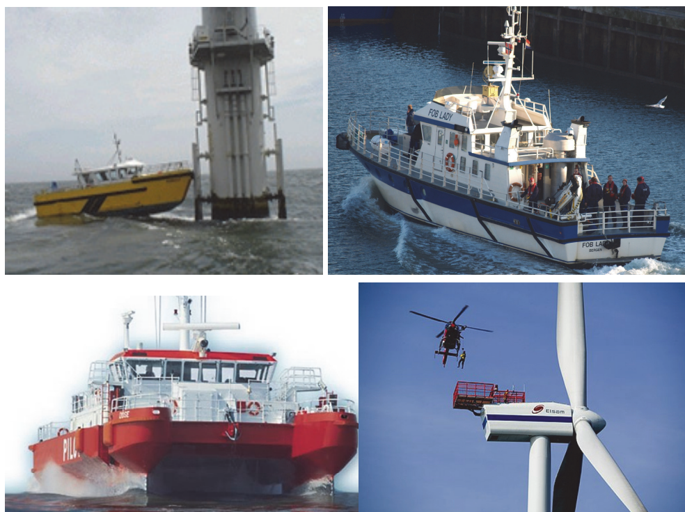
Fig. 4. Examples of transportation and access equipment for maintenance technicians; clockwise: Windcat workboat, Fob Lady, helicopter, and SWATH boat
