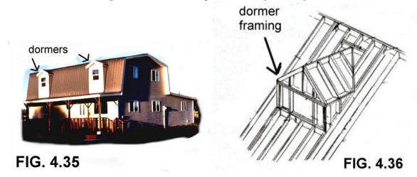
Dormers can be attached to either the side or the top of the roof. The angles can get a little tricky but with a carpenters square and maybe even an angle finder, the job goes quickly and makes a big difference in the overall appearance of the house.
