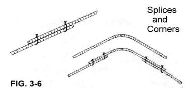
Any place you have rebar that crosses, be sure to tie it up with wire so the cement doesn't force it apart. See **Figure 3-7**.
