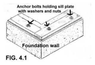
Tighten down the anchor bolts evenly all the way around the foundation to prevent binding which will make an uneven surface.
