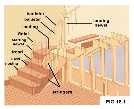
The landing newel will be a really strong support for the rest of the stair railing. It will need to be braced very well. Figure 18.2 shows us how to connect the newel post to the handrail. You will need to drill a hole big enough to get a wooden plug into. A spade bit works best for that. Figure 18.3 shows how to secure the stair treads if you need to.
