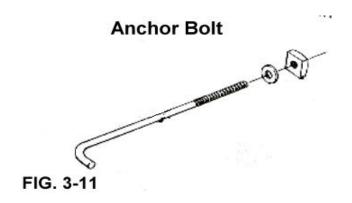
Gravity does a pretty good job holding the house on its foundation, but in unusually high winds, poorly fastened houses have been blown off their foundations. If you forget to put the anchor bolts in the wet cement, you'll hate yourself for a week. While the foundation wall forms are in place and before the cement is poured, mark where the bolts will be
