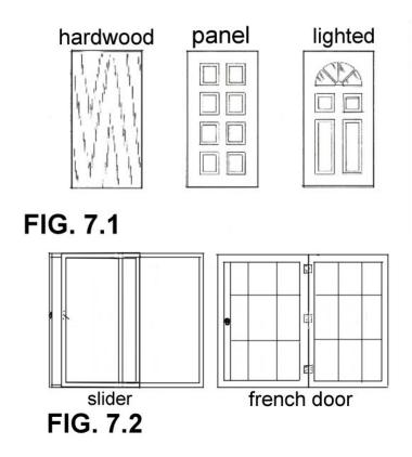
Prefabricated doors come with the jambs, stops, and hinges already mounted so you only have to put them into the rough opening and center them using tapered shims.
