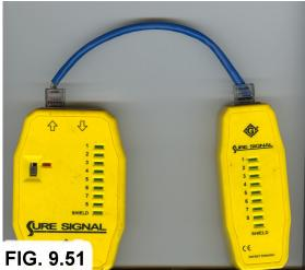
Line testers will test all eight channels on RJ-45 connectors and they are also useful with regular phone line circuits.
