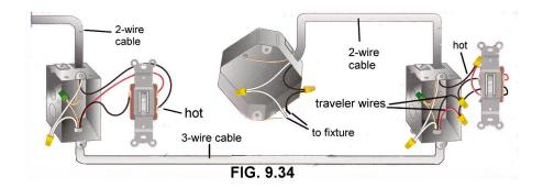
Four-way switches sound confusing, but they are quite simple. Just remember this one thing: four-way switches are always between three-way switches. You can have one light that is controlled from a dozen locations, but you'll start with a three-way switch at the start of the light circuit, place ten four-ways in between, and then end with another three-way switch.
