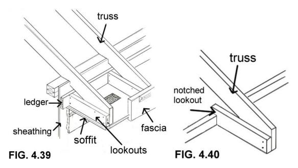
As shown in **figure 4.39**, the cornice is framed in after the wall sheathing is finished, but before the roof sheathing is put on. A ledger is attached to the wall sheathing and runs the distance of the wall. A 2x4 works well for this.
