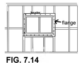
The siding will cover up the flange when the exterior work is done. Keep the windows shut and locked until completely fastened and secure. The windows that don't have a nailing flange are usually a casement type that needs to be fastened from the inside like a pre-hung door. **See figure 7.15**. Nail through the shims for stability. **See figure 7.16**.
