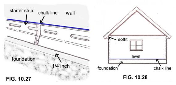
Be sure to leave about ¼ inch gap between starter strips to allow for expansion. Now we can put our first vinyl panel in place. See **figure 10.29**.
