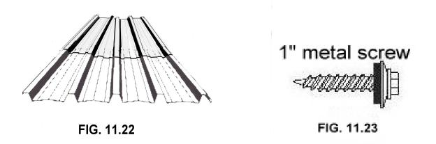
The screws are usually hex head wood screws with a rubber ring. The screw shouldn't be over tightened. The screw is in far enough when the rubber just starts to expand out. **Figure 11.24** shows where the screws should be placed for maximum strength.
