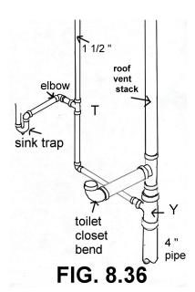
A few decades ago, venting wasn't a major consideration and there was a lot of leniency in the area of wet venting. Trial and error has taken us down learning lane once again. If a vent is full of water or has restricted airflow, an imbalance in atmospheric pressure can suck the water out of traps and also prevent wastewater from draining. Take the time to make sure everything is properly vented.
