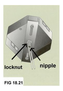
Fans and heavy fixtures will require a connection that uses mounting screws, but small lights as shown in **figure 18.22** and **18.23** only need a nipple mount and are really quick to install.
