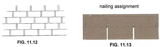
Each 3-tab shingle will need four nails to make it secure. The nailing assignment is manufacturer specific so it should be followed closely. See **figure 11.13**.
