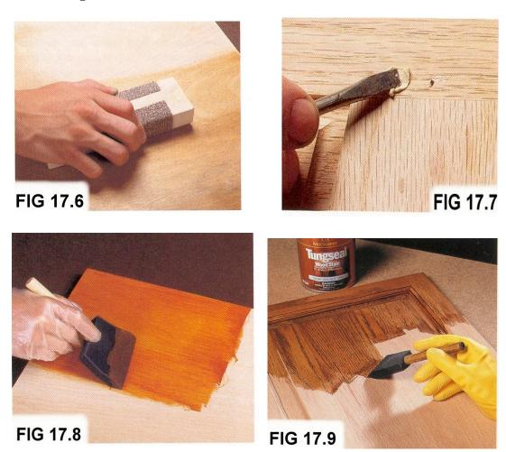
After you get the carcass stained you can stain the doors and let them dry so you can put them on with screws and hinges after the carcasses are hung. The doors should be made of solid wood. It's all right to use veneer on the carcasses, but the doors will have too much movement and the veneer will wear out.
