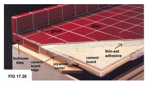
You start with the plywood center. You put a layer of plastic over the plywood. Then put the cement board on with screws. You will need to put cement board on the sides too.
