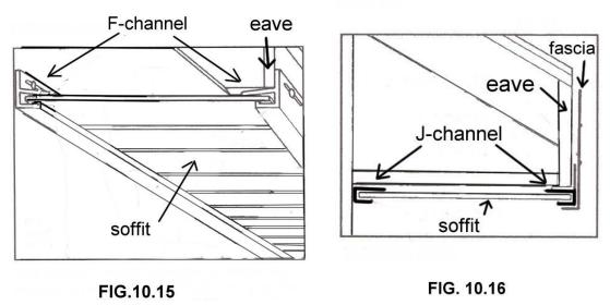
You can see the difference between an open eave as in **figure 10.15**, and an enclosed eave as in **figure 10.16**. The open eave needs the F-channel and the enclosed eave will need to have the J-channel attached.
