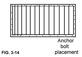
By the way, making your own cement isn't a very practical idea. Have it delivered and poured by the local cement companies. Have a shovel to settle the cement into all the forms so no air pockets remain. You can use a flat board as a screed to make a smooth surface so the sill plate rests evenly on the foundation.
