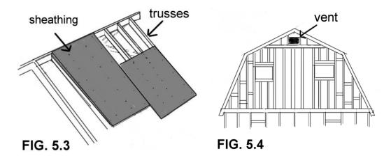
In the attic space, you will need to put a vent in so that there can be airflow to prevent moisture and mold, also to regulate temperatures directly under the roof. The vent is placed above the insulation, but below the truss ridge. It will need to be framed in before the sheathing gets put up. Vent covers can be purchased where you get doors, windows, or siding and retailers will have rough opening measurements. See **figure 5.4**.
