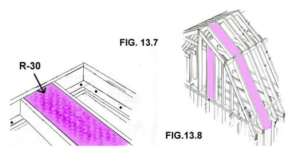
Insulating a Gambrel roof is different than a normal rafter roof because you will need to roll R-30 or R-38 into the rafters as shown in **figure 13.8**.
