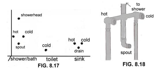
**Figure 8.18** shows how the shower/bath assembly works. You can usually buy this piece as a whole unit that's already measured and ready to install. **Figure 8.19** is how you install the sink shutoffs with compression fittings. The fittings will screw onto the pipe nipple. Copper and galvanized pipe nipple fittings have threaded ends for termination fittings to screw on and for branching off of the mainline.
