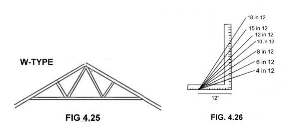
Roof pitch is measured by how much slope is in a 12" measurement. A carpenter's square helps to find the angle. If you measure 4" up on the square and 12" over, you have a 4 in 12 pitch, which is really quite flat. A more common pitch is 6 in 12. That will make a stronger roof and it will shed water faster. Pitches higher than 8 in 12 are usually reserved for special house designs or for areas with very heavy snow and ice loads.
