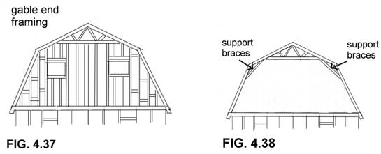
In areas where heavy snow and ice form, a Gambrel roof is a good choice because of the strength. If you have any doubts, you might want to reinforce the knee with support braces. A simple 2x4 works just fine fastened with mending plates or plywood with small nails. See **figure 4.38**.
