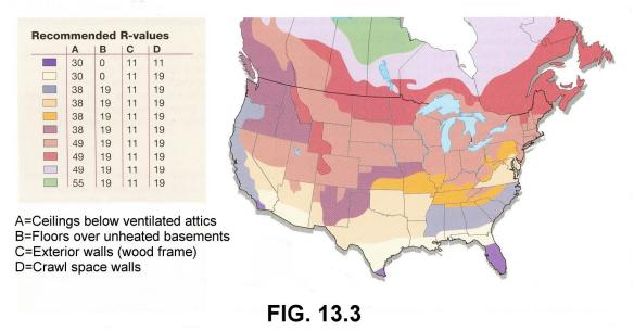
Most codes have a minimum of R-11 for the walls, but if you have 2x6 walls, you will be better off with R-19. It will make a lot of difference in temperature extremes. You can see the R-values according to board thickness in the graph in **figure 13.4**. Some insulation bats have a small flap on the edge to staple so it stays in place. Other rolls might need to be held in place with plastic as in **figure 13.5**.
