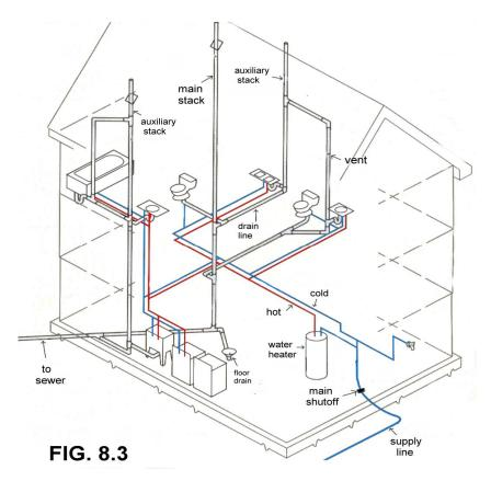
Figure 8.3 shows how the cold and hot lines are routed to the different fixtures. When copper or galvanized pipes are used, this is usually the way it is run. Most often, ½ inch pipe is used.
