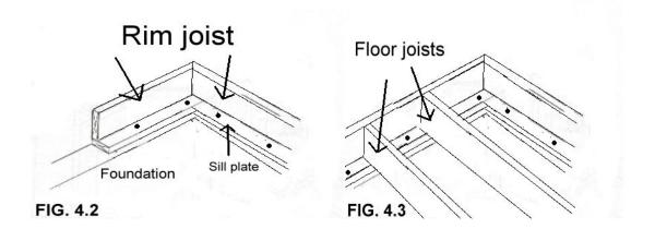
The rim joist is the outside perimeter that the floor joists are attached to. The floor joists are easy to fasten down because you can nail them through the outside of the rim joist. You can use either 2x10's or I-joists for the floor joists.
