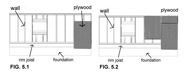
You can offset the sheets for greater strength. The plywood needs to cover the rim joist and sill plate and cover an inch or so of the foundation so water doesn't get in. **Figure 5.2** shows how to nail or screw on the sheets of plywood or wafer-board. The walls will become much more stable once this is finished.
