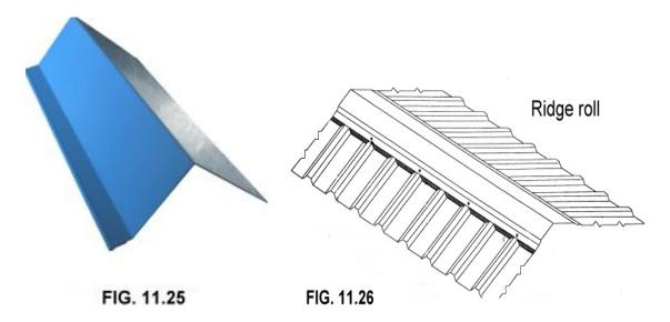
The ridge cap needs to be secured by putting screws in the ridges. That will keep the ridge from bending or buckling in places. You can fill in the valleys under the ridge cap with roof cement to prevent wind and rain from getting in.
