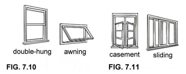
The double-hung and sliding windows are the most popular. Casement windows are usually more expensive. There are also a few of the fixed-frame varieties where the window doesn't open at all. They are mostly used for stairway illumination, skylights and bathrooms. The easiest windows to install are those with a flange. **See figures 7.12, 7.13**.
