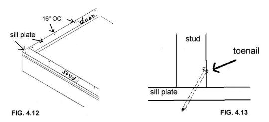
If you opt to put the sill plate down first, then you will attach the wall studs by toenailing. See **Figure 4.13** Otherwise, you can pre-build the walls in 8 ft sections and stand them up and then nail them to the floor. You need to nail into a floor joist for strength. If you are using 2x6's for walls, then you will probably want to build in 8 ft sections because of the weight when standing them up. **Figure 4.14** shows a complete wall.
