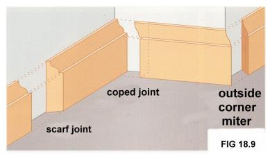
This is how the trim pieces are cut to fit together. There is the scarf joint that joins
