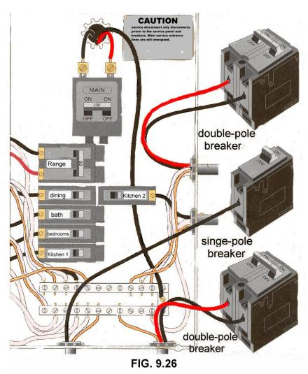
The breakers just pop into place as they attach to the hot bus bars. You will need to label each breaker so you don't forget which circuit it is.
