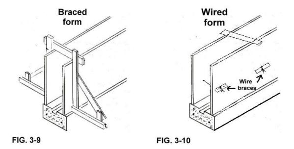
In **Figure 3-10**, we see how to use wire by drilling small holes in the boards or plywood, running wires through and twisting them around wood pieces. Once the cement is hard, you can cut the wires or even break them off with a hammer so you can release the forms.
