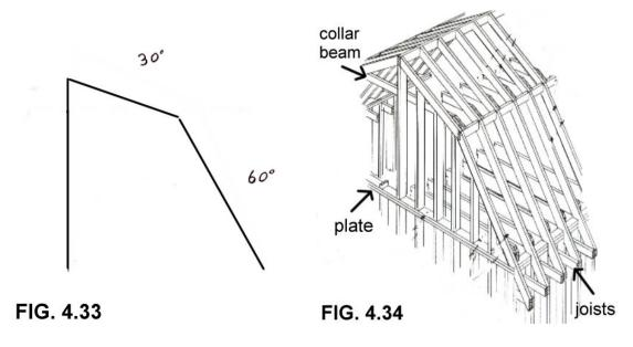
As illustrated above, in **figure 4.33**, a 30/60 slope isn't difficult. It can just about be attained by guesswork alone. It is important to distribute the weight from the ridge to the knee. Also a collar beam will be necessary and it will help relieve pressure from the sides of the roof. Most gambrel houses have dormers to help improve the looks from the outside and to provide a view and sunlight on the inside.
