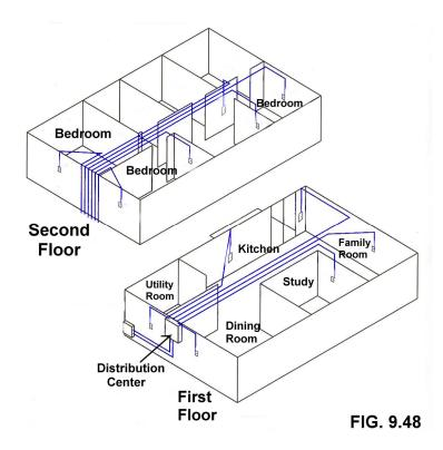
It is always a good idea to run all the communication cables together. They're easier to manage that way and you can keep everything organized all in one strand. The terminations for the RJ45 connectors are color-coded making it easier to keep the wiring order consistent. The wires each fit into a slot that cuts through the plastic coating and make a solid connection with the copper wire inside. See **figure 9.49**.
