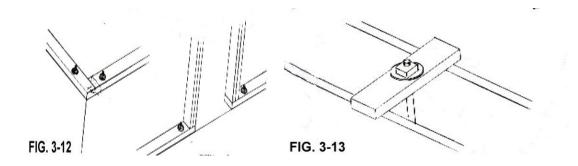
Also, it's a good idea to hang the anchors using a piece of 2x4 because the board is the same thickness that your sill plate will be as shown in **Figure 3-13**. Try to plan ahead before laying out the spacing of the anchor bolts so you don't put one where a joist will be because the floor joists will rest upon the sill plate. Check out **Figure 3-14**.
