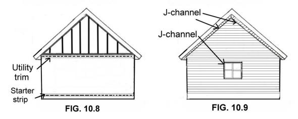
You will use J-channel on gable ends, but also around windows and doors. The vinyl panels will tuck neatly inside the J-channel. A lot of J-channel will be used because of all the windows and doors in a home, but it's very inexpensive and it's extremely easy to work with.
