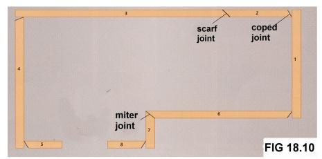
trim pieces in a line. There's the coped joint that's used for inside corners, and there's the outside miter joint for outside corners. This is the simplest way to do baseboards.
