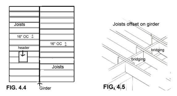
It helps to offset the joists over the girder. You also need to add bridging between the joists for stability as well as fire blocking as seen in **figure 4.5**.
