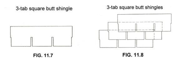
The most important thing to remember about shingles is that they need to be offset so that the tabs don't line up. So we need to have a starting point to begin. We already know that we want to start at the bottom of the roof and work our way up, but some contractors like to start at one end of the roof while others like to make a centerline and start from there. Measure the halfway point and snap a chalk line for a reference point. See **figure 11.9**.
