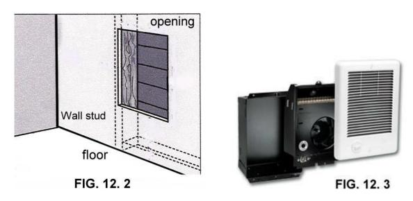
The wiring for these heaters is easy as well. For the 240-volt heaters, you will want to use a 30-amp breaker at the breaker box, and 10-2 Romex with both black and white wires as hot. See **figure 12.4**. These heaters should be placed on interior walls for the best efficiency so they aren't trying to heat cold air of an outside wall.
