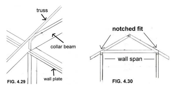
There is a notched fit on top of the wall plate so the truss can extend beyond the wall about 16" to create the eave. Some call this angle cut a bird's mouth. It helps the truss fit tightly into place before it is nailed. See **figure 4.31**. You can fasten the truss by either toe nailing it in place or by using truss fasteners. See **figure 4.32**.
