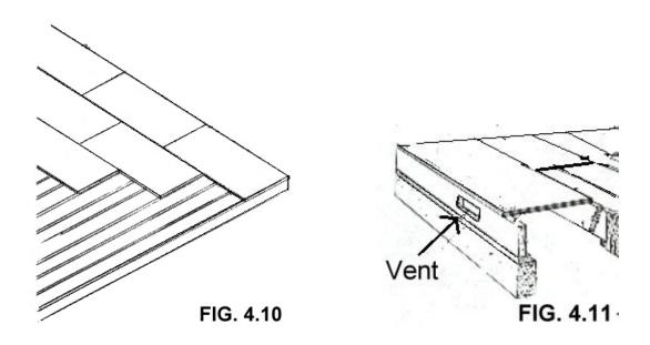
You will also need to cut a vent hole in the rim joist about every 15' or so to increase airflow and prevent the joists and floor from rotting. See **figure 4.11**
