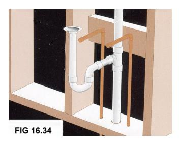
**Figures 16.33** and **16.34** show how the p-trap assembly is connected to the septic line. The sink will next need to be put into a cabinet. The one-piece sink and counter top is very popular these days. See **figure 16.35**
