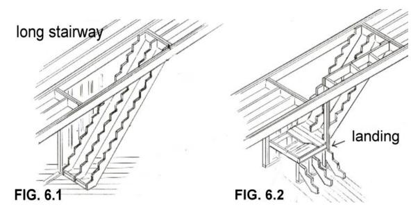
Basically, your stairs have to reach your second floor and you have just so much floor space to do it with. If you look at it that way, it's just a matter of deciding how wide to make the treads, stepping off the number of treads, and then dividing the height of the stairway by the number of treads. That gives you the riser height. There is a little more to it than just that, but there are a few tricks to help with the calculations.
