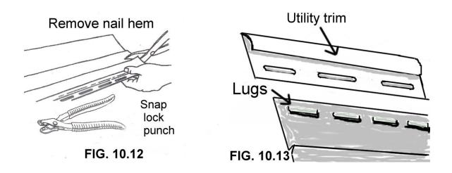
Before the vinyl panels can be put on, all trim accessories have to be put in place. That includes flashing, soffit and fascia, J-channel, F-channel, utility trim, starter strip, inside corner posts and outside corner posts.
