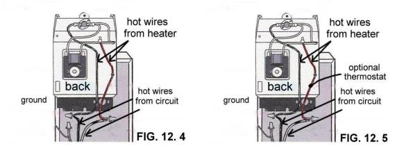
You can use 12-2 Romex, but 10-2 wire will tolerate higher wattages without getting hot. That way if you want to put in a larger heater in the future, the wiring will support it.
