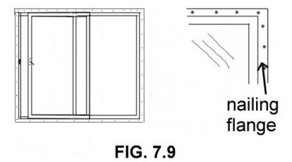
You can use much shorter screws on these kinds of doors. 1" brass screws work really well. Sliders have to be perfectly level and square or the sliding mechanism binds and the door will be hard to open. Even the heaviest of slider doors should be able to be opened by a small child. The sliding door moves on a rail. This rail may need to be polished on occasion with silicone spray. The door lock on a slider will be a small lever with a hook that catches the striker latch when engaged.
