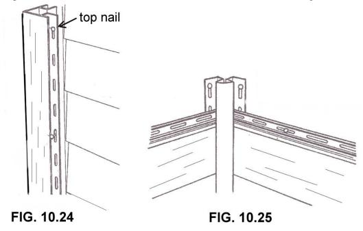
When putting the corner posts on, you need to leave a ¼ inch gap between the top of the corner post and the eave or soffit. The corner posts will also extend down below the starter strip by about ¾ inch. That will make a neat appearance once the vinyl is in place. After the corner posts are done, you can put the external outlet fixtures on. These are prefabricated vinyl fittings for outlets, lights, spigots, dryer vents, etc. See **figure 10.26**.
