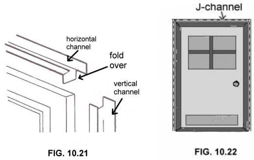
After the flashing, comes the installation for the J-channel around windows and doors. The top piece of J-channel needs to overlap the side pieces as shown in **figure 10.21**. This helps keep water from getting in. **Figure 10.22** shows a door lined with J-channel. The windows are the same.
