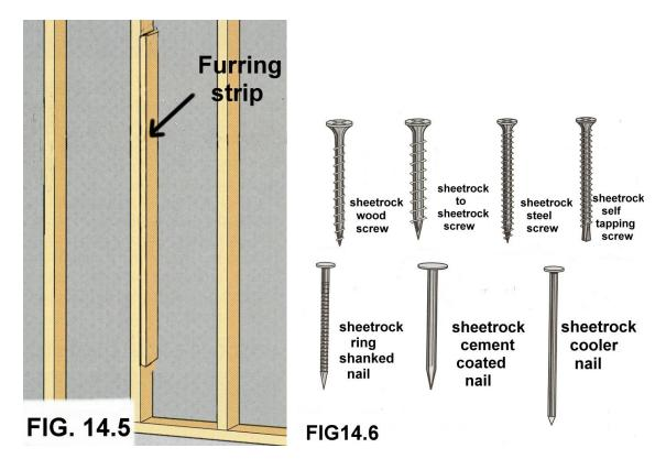
These are screws and nails made solely for securing sheetrock. The nails need to be driven in just lower than the sheet's surface, but not deep enough to break the paper. It's easier to cover the nail heads that way. It requires a special hammer as shown in **figure 14.7**. If you choose to use sheetrock screws, make sure that you don't screw them in too deep.
