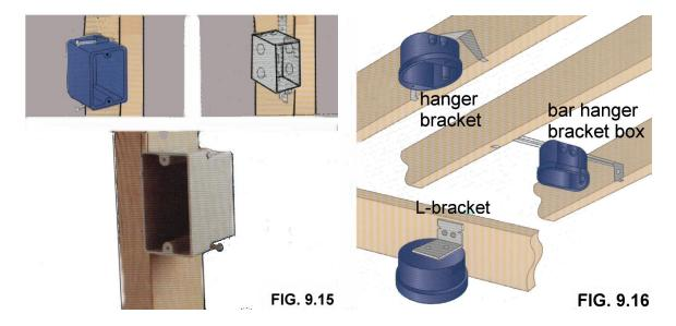
The bar hanger junction box gives more support than a normal hanger bracket. See **figure 9.16**.
