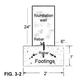
This gives a good idea about the dimensions and how to put the rebar in so it gets completely covered. You can also use "rebar chairs which is a little wire frame to hold the rebar in place.
