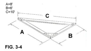
After you get a good square measurement on the outside of the footings form, start the inside and measure the width of the footing.
