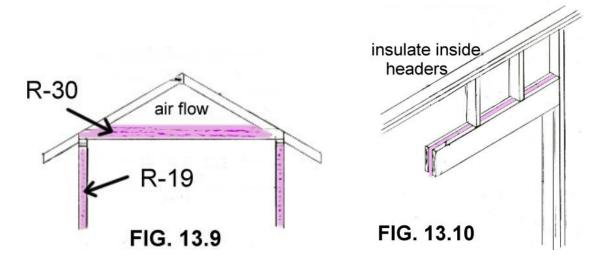
There are a few areas that often get overlooked when insulating. One of those areas is inside headers and between rough openings for doors and windows. See **figure 13.10**. Also behind outlets, switches, and any place where there are openings in the sheetrock.
