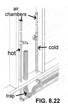
a hot and cold line also. **Figure 8.22** shows how to run the hot and cold lines. These lines are usually brought together in a recessed wall box with spigots to hook up the washer supply lines as well as a waste line for the washer to pump out dirty water. **See figure 8.23**.
