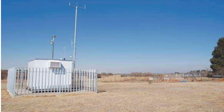
Fig. 6. Measuring station for taking particulate matter measurements Source: State of Air Report (2005)
