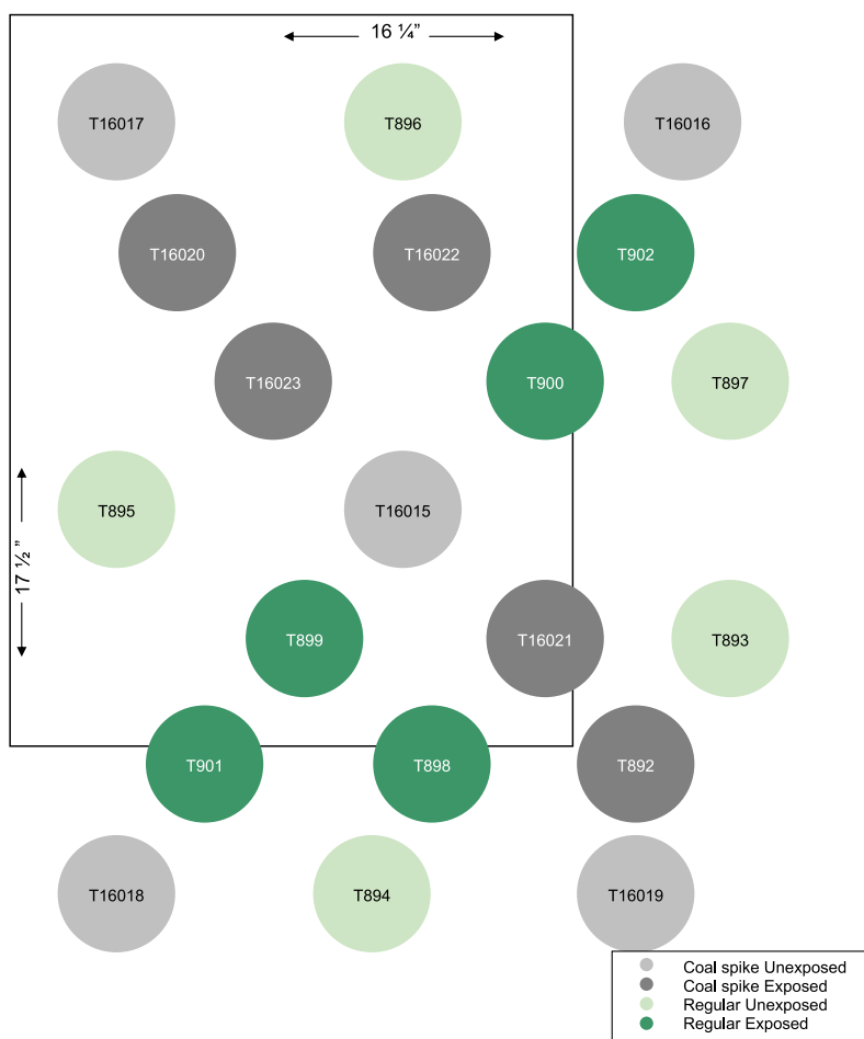
Fig. 1. Total Dust Fall Method Validation - Field Performance Study/Filter Placement Schematic
