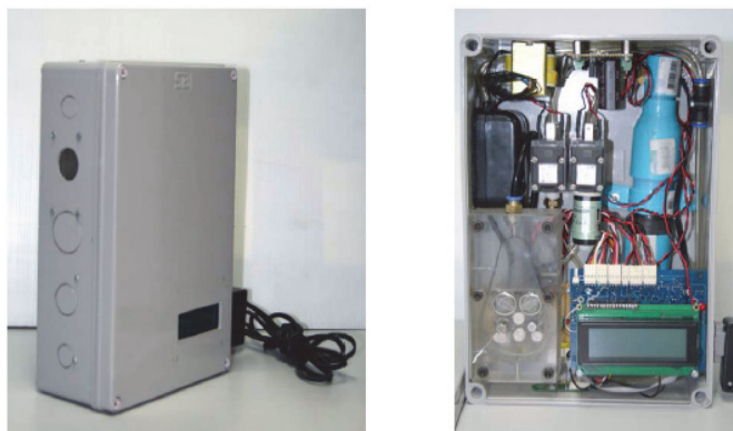
Fig. 18. Photographs of a wireless E-nose based on ZigBee wireless network (Pogfay et al., 2010).
