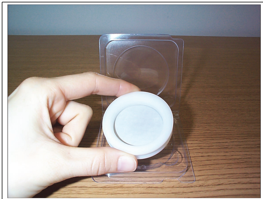
Fig. 2. Teflon Filter (47mm) Oil Coated in Sampling Cassette with Shipping Container (Ready for Field Use)
