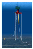
Fig. 1.1 The static configuration of SCR
