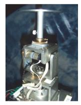
Fig. 2. Rotational motion simulator using z-y-z Euler angles.
