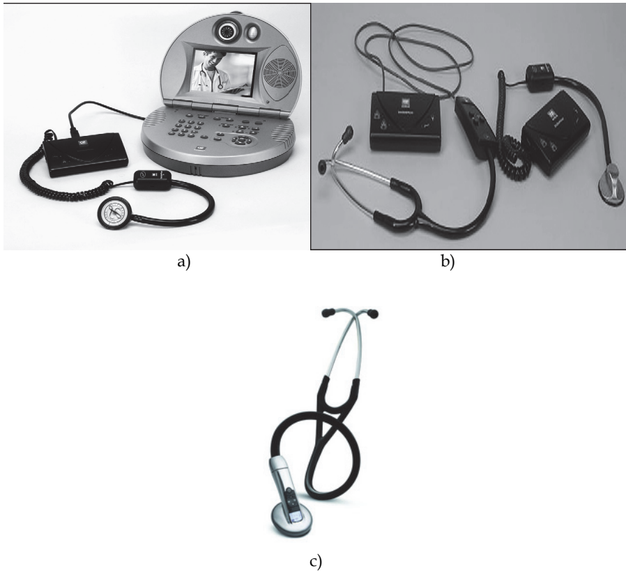
Fig. 6. (a and b) Commercially available tele-stethoscopy system from Aethra and (c) Digital stethoscope
