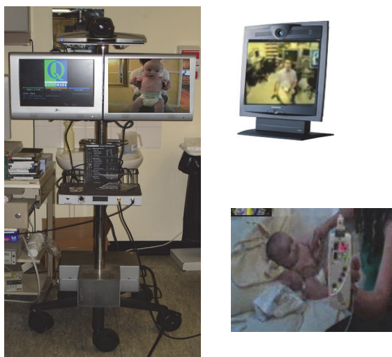
Fig. 5. Telemedicine hardware needed for hospital-home videoconferencing. What the doctor sees and what the family sees
