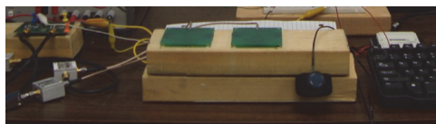
Fig. 11. A picture of the 2nd generation sensor with discrete components (PC not shown)
