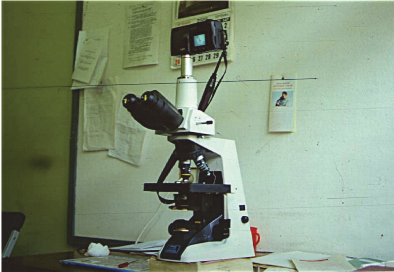
Fig. 10. The basic instrumentation for static telepathology is simple and inexpensive: a trinocular microscope coupled with a digital camera and a web connection.
