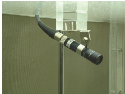
Fig. 9. Microcamera fixed on the ceiling of the tunnel at the downwind end.
