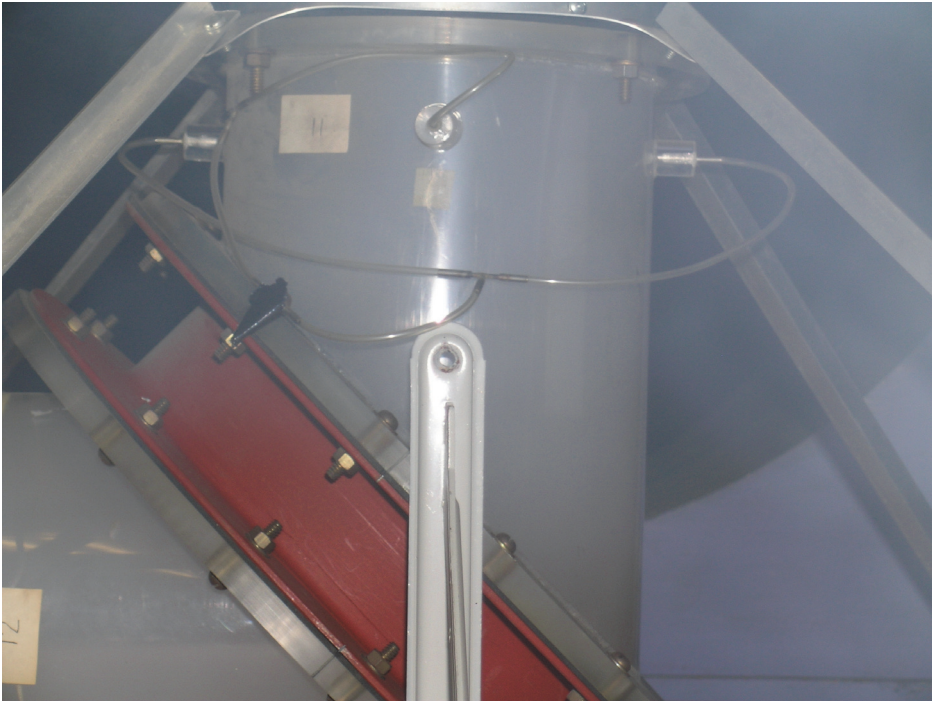
Fig. 22. Smoke flow visualisation at the intake.
