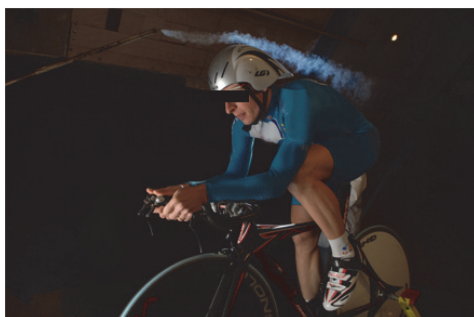
Fig. 13. Smoke stream around a time trial cyclist and his equipment (Wind tunnel of Marseille, France).
