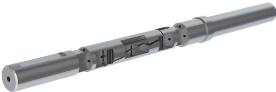
Fig. 1. Internal balance example. Image courtesy of STARCS.
