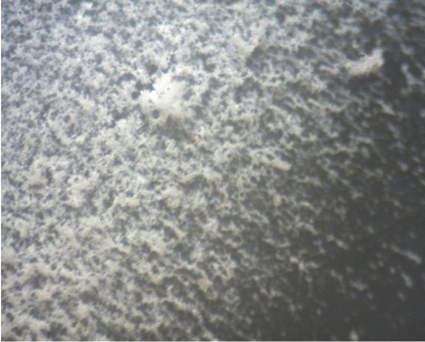
Fig. 14. Aggregated quartz grains ( <2\mu\text{m} ) deposited on an upward facing surface after wind tunnel aerosol exposure.
