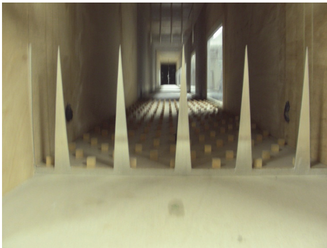
Fig. 8. Turbulence spires and roughness array for a nominal friction speed of 0.4 m/s.
