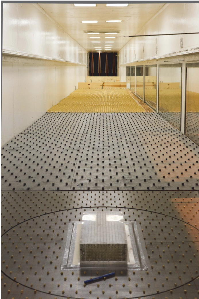
Fig. 1. Meteorological wind tunnel, Wind Engineering Laboratory, Colorado State University. Model and turntable are in the foreground, and spires are in the background (courtesy of Professor Bogusz Bienkiewicz; photo by Gregory E. Stace).
