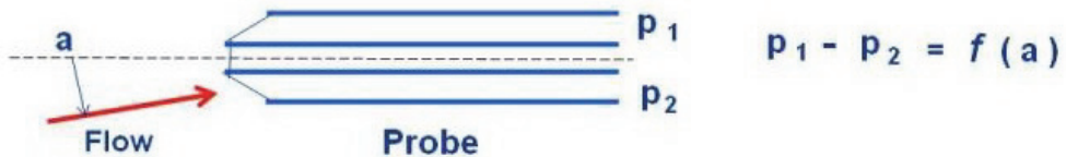
Fig. 3. Vertical cut of three tubes showing the leading edges and the angle determination concept
