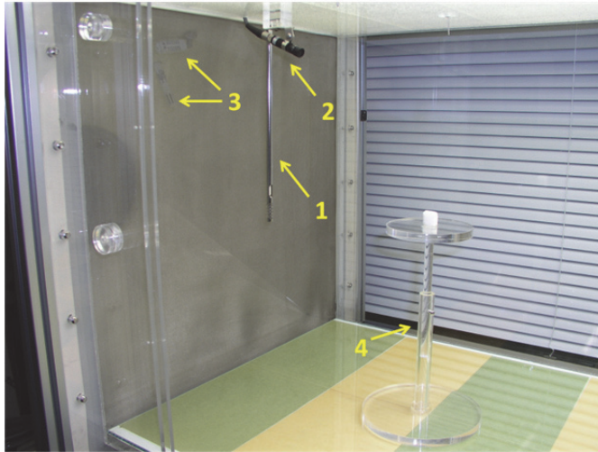
Fig. 5. Downwind end of the tunnel. 1: anemometer; 2: VTR camera; 3: thermometer and hygrometer; 4: platform to release insects.
