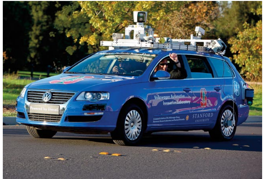
Junior, a robotic Volkswagen Passat developed by Stanford University, is capable of navigating urban environments autonomously. It can select its own routes, perceive and interact with traffic, and execute urban driving skills including lane changes, U-turns, and parking. The vehicle successfully finished and won second place in the DARPA Urban Challenge. (Stanford University)
