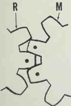
Fig. C1-9 - Diagram showing crankshaft (R) and camshaft (M) timing gear marks.
