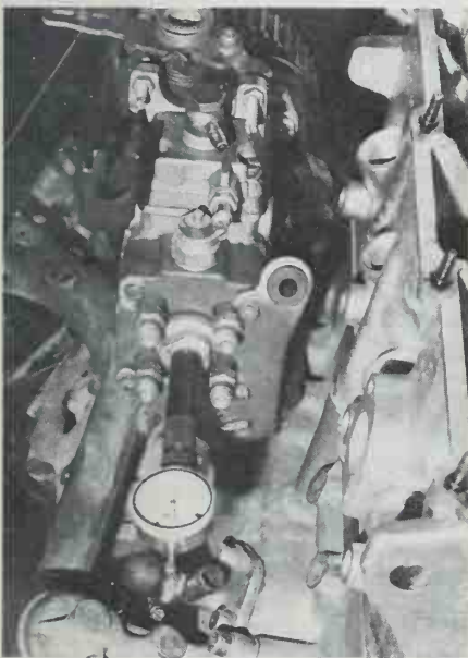
Fig. V1-3—View showing installation of dial gage in injection pump for injection timing. Injection lines may remain connected.
