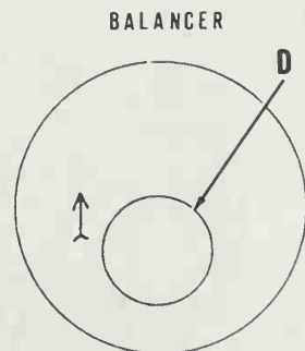
Fig. L4-17—Arrow on piston crown should point towards injection pump and depression (D) should be near injectors.
