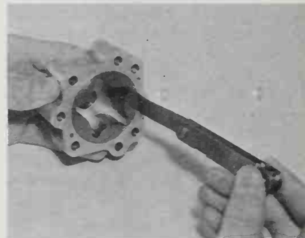
Fig. K3-23—Measure clearance between outer rotor and oil pump body as shown. Desired clearance is 0.11-0.19 mm.
