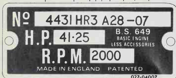
Fig. L1—View of typical engine identification plate used. To insure use of proper parts and specifications, use complete number.
