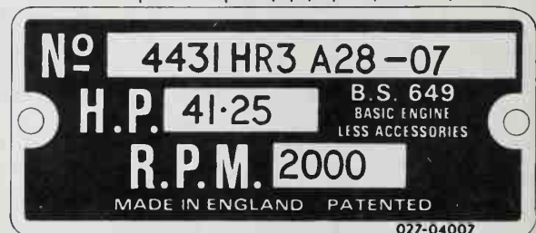
Fig. L25—View of typical engine identification plate used. To insure use of proper parts and specifications, use complete number.
