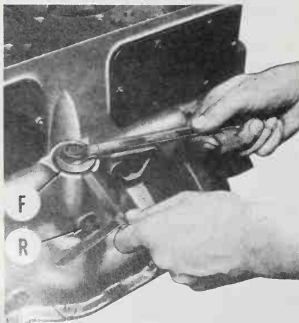
Fig. P1-25—Measure clearance between flange screw (F) and boss as outlined in text. Taper screw (R) holds oil pump in block.
