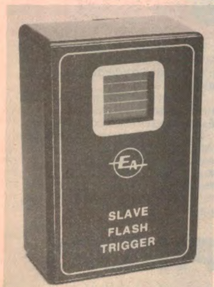
The completed prototype. A thin piece of glass should be glued over the cutout to protect the solar cell.
