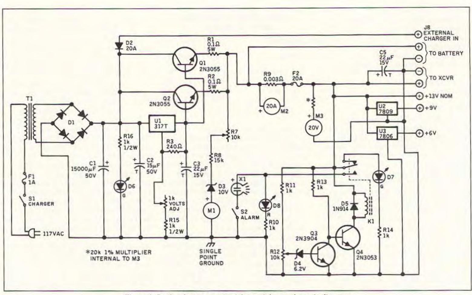
Figure 1. Backup battery monitor/charger/alarm schematic diagram.
