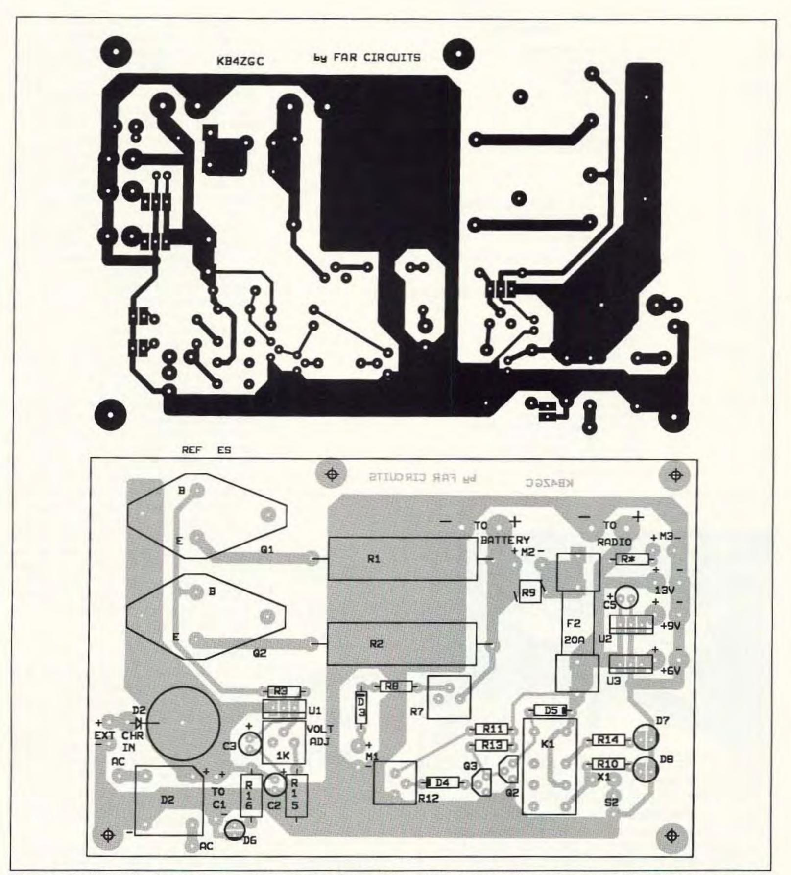
Figure 2. Circuit board and parts placement for the Backup Battery Monitor/Charger/Alarm. Note: If transistors Q1 and Q2 are mounted on the PC board, they must be heat-sinked. The transistors may be external to the board and wired back to the PC board.
