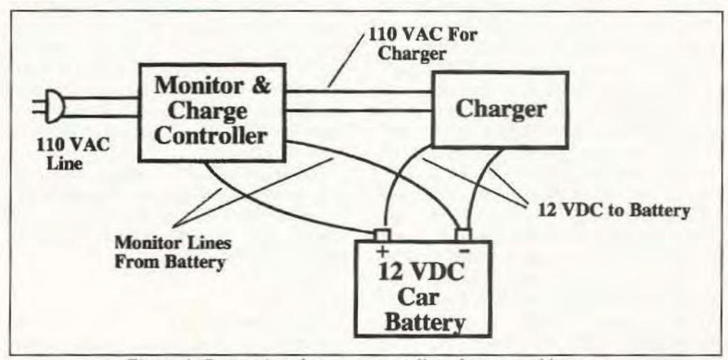
Figure 4. Connections between controller, charger and battery.
