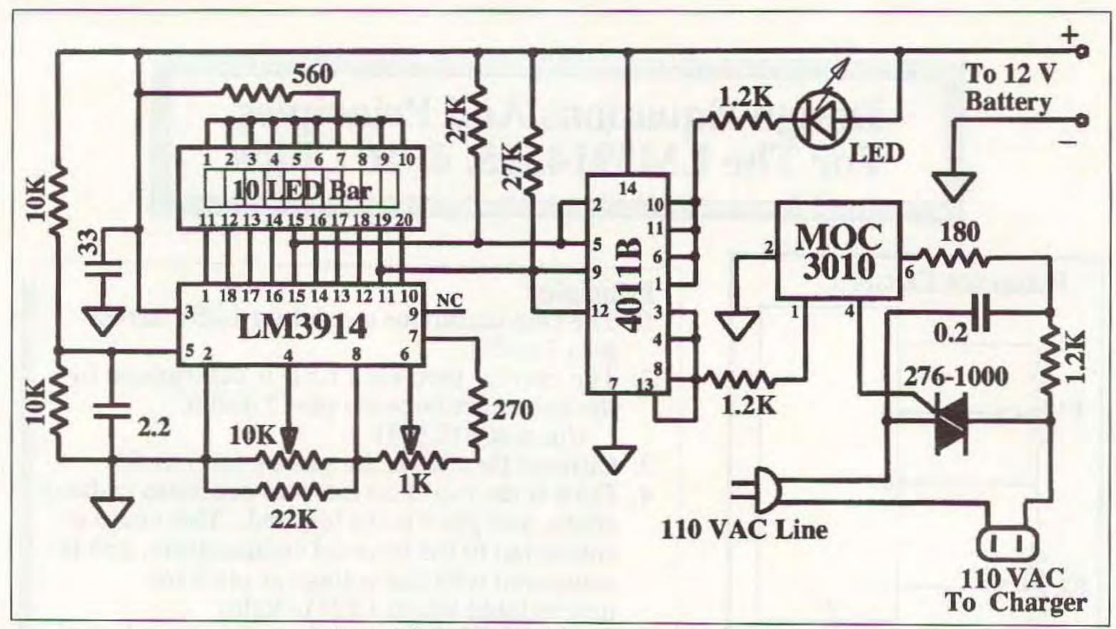
Figure 1. Battery monitor and charge controller schematic.
