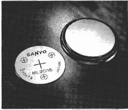
FIG. 8—RECHARGEABLE lithium cells are intended principally for maintaining the contents of solid-state memories.
