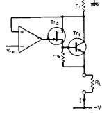
• Mse f.e.t. 2NS457 to drive the bipolar transistor. Absolute measure nent of current through R<sub>1</sub> and emitter currents of Tr<sub>1</sub> now indicate a variation of less than 1%. R<sub>1</sub>: 1.1kΩ, R<sub>3</sub>: 100. Ver dyasted to give load current of 2mA. R<sub>4</sub> varied from 4.7kΩ (nax) down to 10. Current change within 0.01%.
