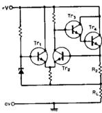
If regulator is placed some distance from the d.c. supply filter, a capacitor of about  $0.1\mu\text{F}$  may be required between terminal 1 and ground to prevent h.f. oscillation.
