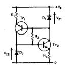
Typical performance Minimum terminal p.d.  $\sim V_{Z_2} + V_{Z_1} - 0.5V$ Constant current  $V_{\rm Z_2} - 0.6$  $R_3$  $R_1$ Tr<sub>1</sub>: 2N2702 Tr<sub>2</sub>: 2N3707
