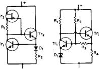
Tr<sub>1</sub>: n-p-n germanium transistor (OC139, 2N1302, 2N1304, 2N1306, 2N1308).
