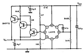
regulator against excessive power dissipation should the load short-circuit, and limits the current to about 0.5A. Limiting starts when the voltage across terminals 1 and 8 exceeds +0.4V, and depends on the potential differences across Ritmit and R<sub>4</sub>. This critical voltage increases the positive bias on a transistor which therefore conducts harder and steers current away from the first transistor of the series element, andhence the load current decreases.
