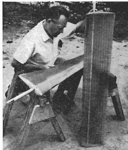
Lightweight rotor blades, based on a sophisticated airfoil for highest efficiency, are checked by Midwest Editor E. F. Lindsey who helped Meyer with plans (left).
