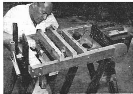
Top view of carriage shows batteries, in storage tray, and voltage regulator. Batteries serve triple purpose: Energy storage, alternator excitation, counterbalancing.
