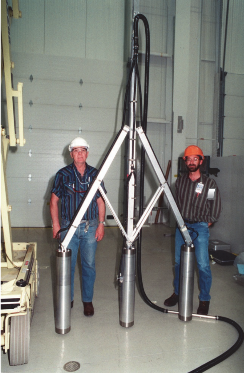
Fig. 3. Multi Detector Basin Scanning Array for INTEC-603.
