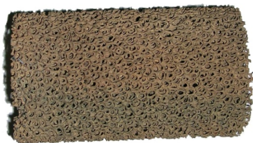
Fig. 8. Structured steam reforming catalyst
