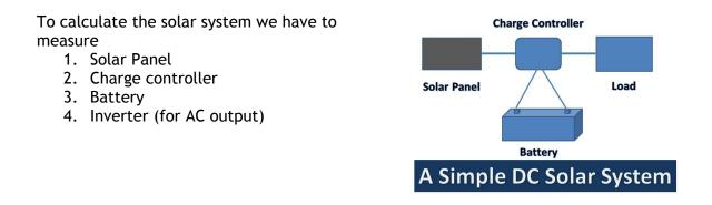
Now if a subscriber wants to setup <u>a solar system for 2 bulbs and 1 fan. (12 volt DC)</u> (1 bulb=10 watt, 1 fan=20 watt) then the total load
