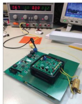
Figure 31 – EMI mitigation using a CM choke and “finger shield”.
