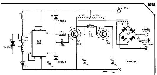
This inverter circuit can be used to power electric razors, stroboscopes and flash tubes, and small fluorescent lamps from a 12 volt car battery. In contrast to the usual feedback oscillator type of inverter, the oscillator of this inverter is separate from the output stage, which allows easy adjustment of the oscillator frequency to suit different applications.
