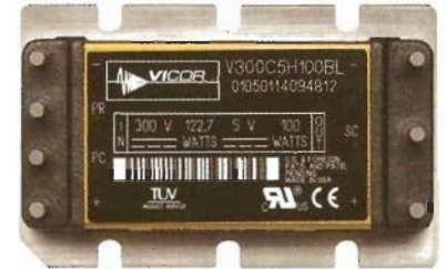
Fig. 1. A commercial dc-dc converter that employs zero current switching.
