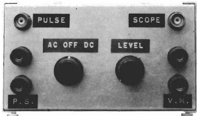
2. All packed up and ready to go. Complete electronic load circuit, including the 9-volt battery that powers it, is housed in a standard 3-by-2-by-5 1/4-inch aluminum box. Connectors can be seen.
