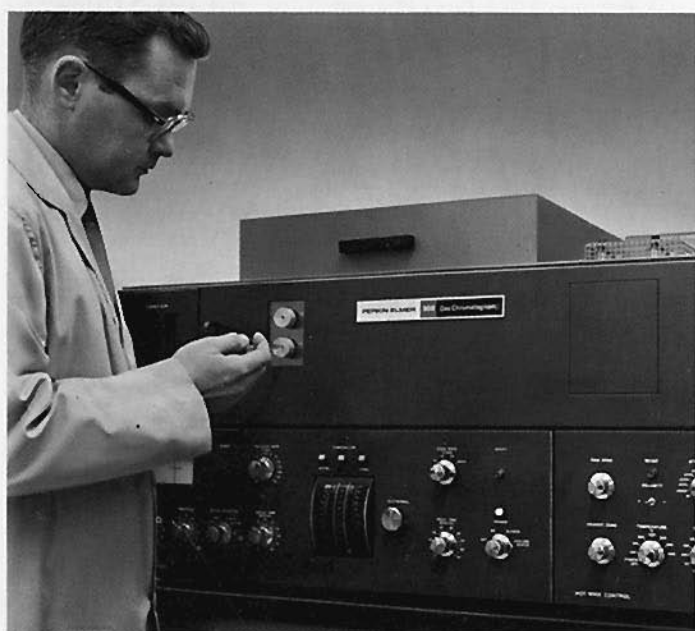
Chianti, vintage 1957, is introduced into the gas chromatograph. Comparison of differences in trace components on the chromatograms may be related to differences in relative quality of individual vintages.
