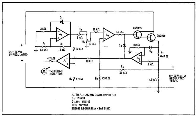
Op amp regulator. An unregulated 26-volt source becomes a 1-ampere 0-to-20-V supply regulated to within ±0.02% by a simple quad operational amplifier. Input can vary between 24 V and 28 V, and quiescent current is less than 10 mA. A light-emitting diode gives an overload indication, the level of which depends on the value of resistor R<sub>8</sub>. Single power Darlington can replace the two transistors.
