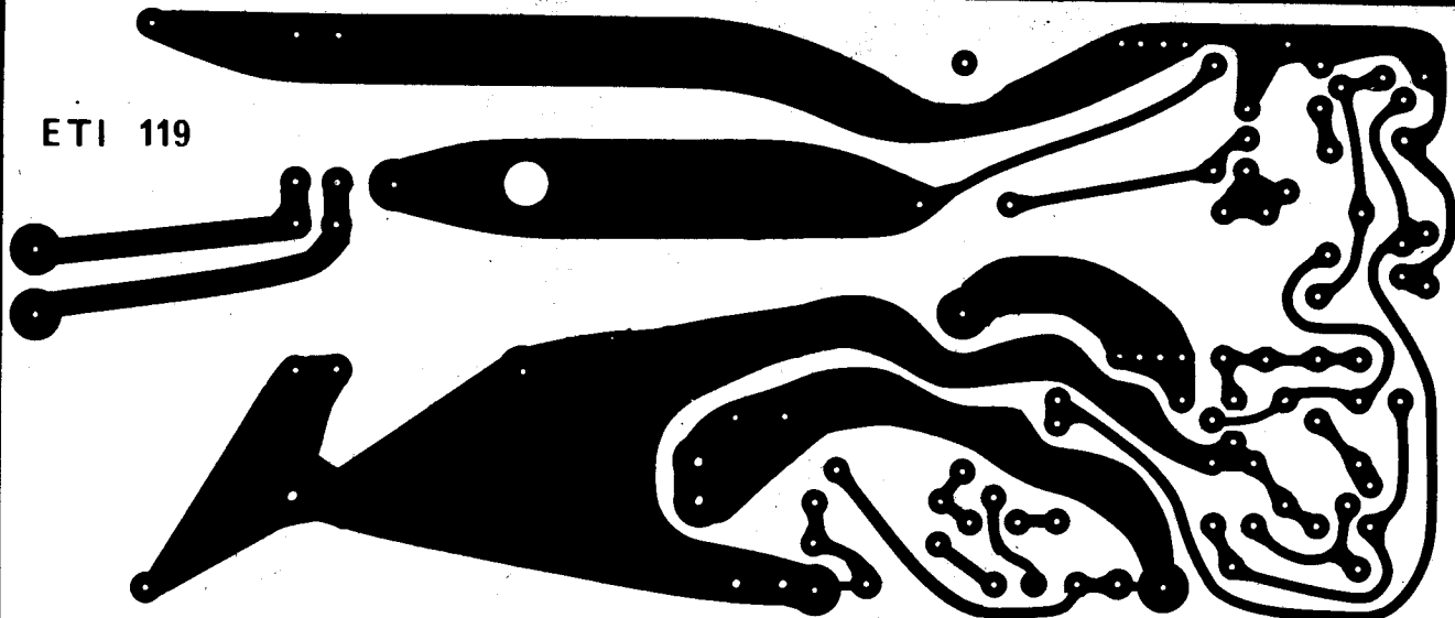
Fig. 4. Printed circuit-board layout. Full size. 178 x 78 mm.
