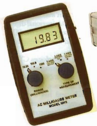
Figure 4 Inductive-sensor instruments can measure only ac fields (courtesy AlphaLab).
