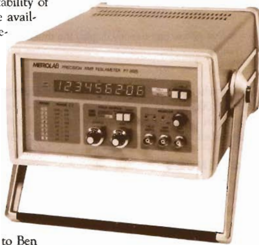
Figure 8 This NMR gaussmeter offers 5-ppm accuracy but can measure only dc or very-slow-ac fields (courtesy Metrolab) and comes with an optional PDA (courtesy GMW Associates).
