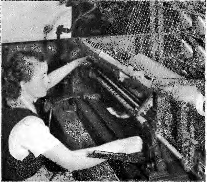
FIG. 33. Winding 20 coils in multiple machine: layer paper at right.
