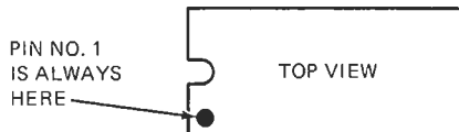
FIG. 1—FINDING PIN 1 of a dual-inline-package (DIP) IC is easy. Just look for the notch in one end as shown here.
