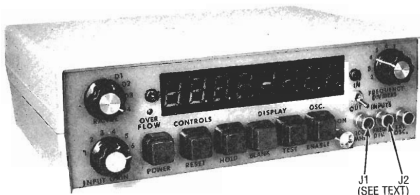
FIG. 6—THE FINISHED FREQUENCY COUNTER, shown in display-test mode, with all digits and decimal points lit. J1 and J2 are wired together, but one is unnecessary (see text).
