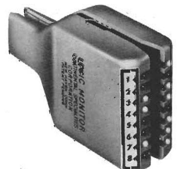
CSC's 16-LED Logic Monitor clip displays states of all IC pins at once.
