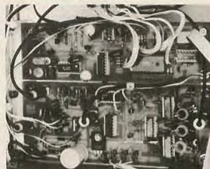
FIG. 17—CONTROL AND VCO BOARDS are mounted side-by-side. Switch board, not seen here, sits above coils at lower right. BCD thumb-wheel-switches are visible at top of photo.
