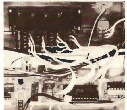
FIG. 8—SWITCHES AND CONTROL BOARD mounted in case. Usefulness of ribbon cable is obvious.
