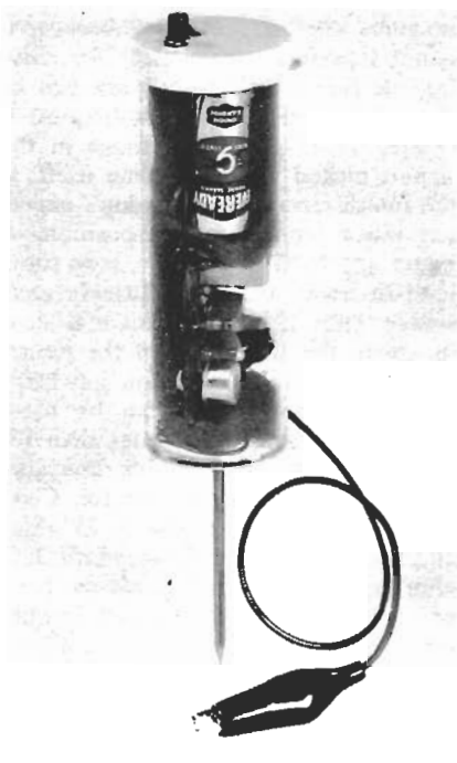
ANOTHER VIEW shows how parts are cushioned with pieces of foam rubber.
