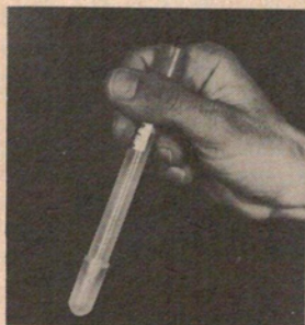
Store the pH electrode with its tip soaking in distilled water, use the protective shield and rinse with distilled water between measurements.
