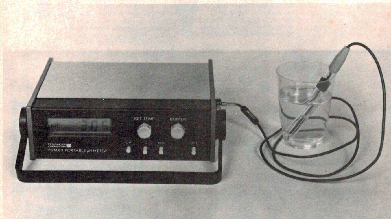
A high quality portable pH meter with a liquid crystal display that directly indicates the pH of the solution under test.
