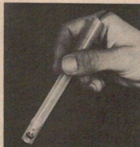
Store the pH electrode with its tip soaking in distilled water, use the protective shield and rinse with distilled water between measurements.
