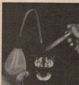
Store the pH electrode with its tip soaking in distilled water, use the protective shield and rinse with distilled water between measurements.
