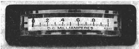
Shallow-meter design of Hoyt Electrical Instrument Works.
