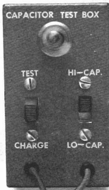
Completed electrolytic tester.
